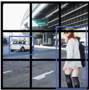
Figure 5.53: Non-max suppressed outputs pseudo-algorithm.
