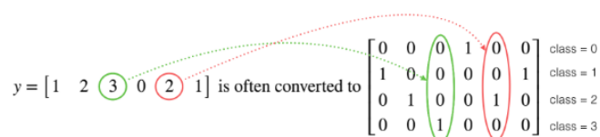
Figure 5.9: An example of one-hot encoding with 4 classes.
